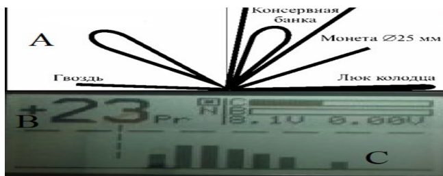
Figure 2 – Example of visualization: A) hodograph; C) the number of VDI; C) Sinograph
