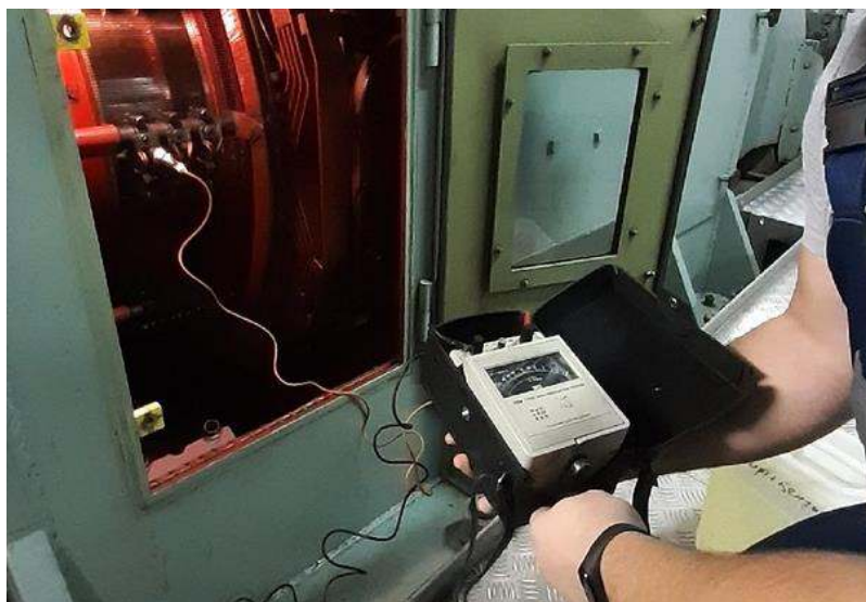
Figure 3 – Measurement of insulation of the collector mechanism
