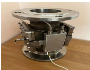
Fig. 6.- Appearance of measuring chamber and primary converting unit.
