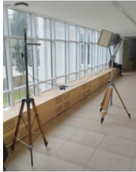
Fig. 4 — Photograph of the experimental setup for determining the antenna's axial ratio
