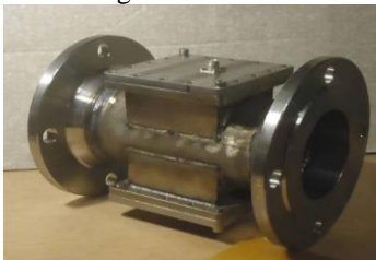
Fig. 2. A prototype of the measuring chamber of the microwave moisture meter of petroleum products.
